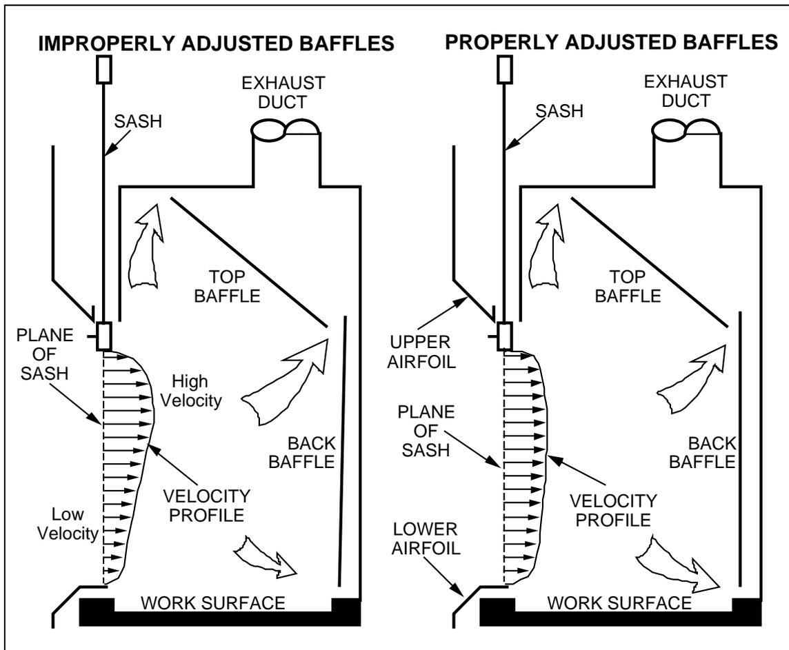
Figure 3: Baffle Optimization
