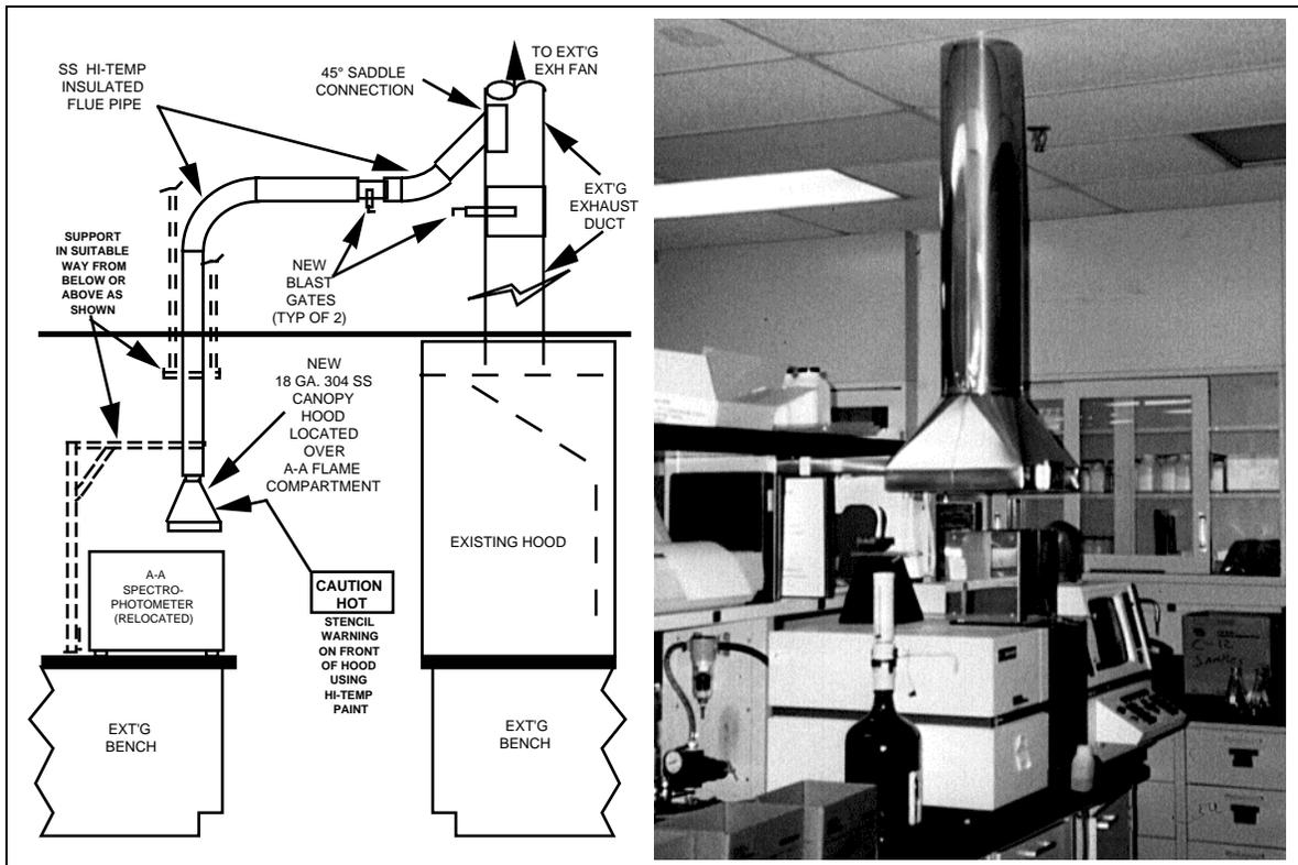
Figure 7: Atomic Absorption Spectrophotometer Hood
