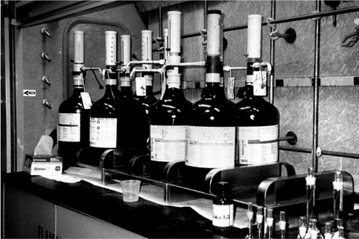
*Figure 8: Typical Reagent Bottle Rack*
